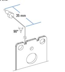
**9** Insert the capillary into the hole between fixing screw and the inlet fitting.
