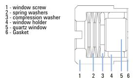
Figure 74 Orientation of Spring Washers
