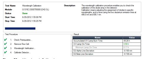
Figure 59 Wavelength Calibration
