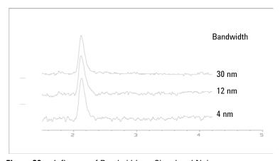
Figure 36 Influence of Bandwidth on Signal and Noise
