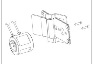
11 Re-install the flow cell and connect the capillaries to the union holder.
