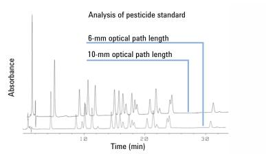
Figure 33 Influence of Cell Path Length on Signal Height
