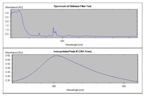
Figure 52 Holmium Oxide Test (Signal)
