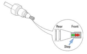
Figure 13 Capillary fitting
