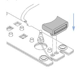
7 Fix the new heat exchanger to the clamp unit and the heat exchanger to the cell body.
