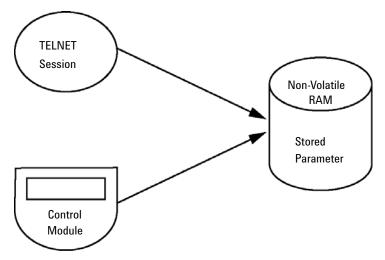
Figure 98 Manual Configuration (Principle)
