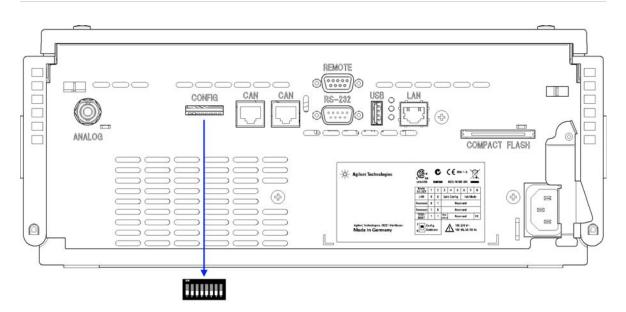
Figure 83 Location of Configuration Switch (example shows a G4212A DAD)
