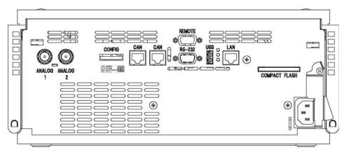
Figure 81 Rear View of Detector
