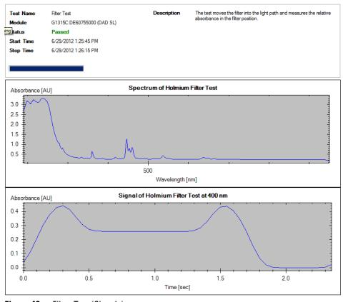
Figure 48 Filter Test (Signals)
