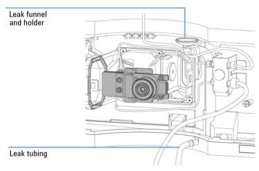
Figure 62 Replacing Leak Handling System Parts
