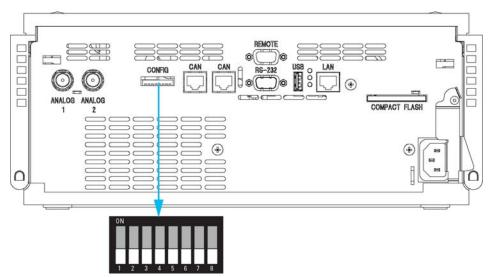
Figure 86 Location of Configuration Switch
