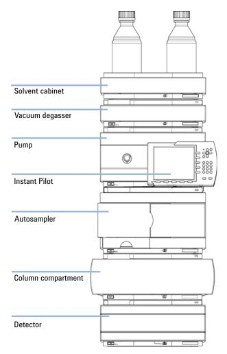
Figure 3 Recommended Stack Configuration for 1260 Infinity (Front View)
