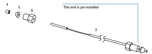
Figure 79 Inlet Capillary (Column-Detector) Parts
