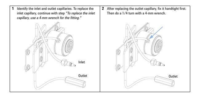
Replacing Capillaries on a Standard Flow Cell
