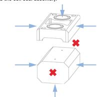
**8** Slide the quartz body completely into the cell body to the front stop (use for example a toothpick).
