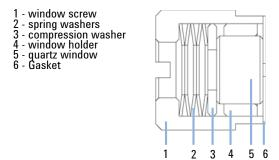
Figure 72 Orientation of Spring Washers
