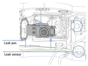
Figure 61 Observing for Leaks
