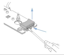
**6** Carefully insert the I.D. tag into the new heat exchanger. Shown is the default orientation. See Note at the beginning of this section.
