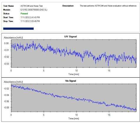
Figure 53 ASTM Drift and Noise Test
