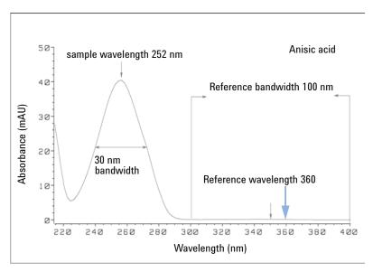
Figure 35 Optimization of Wavelength Setting
