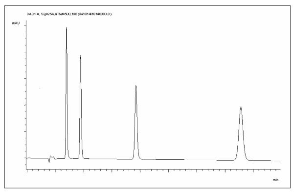
Figure 14 Typical Chromatogram with UV-detector
