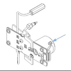
**9** Check for a centered holder vs. hole. If required adjust with the holder screws.
