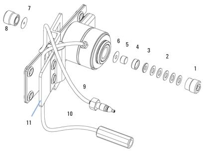
Figure 65 Standard Flow Cell Parts
