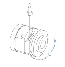
Replacing Capillaries on a Standard Flow Cell
