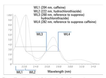
Figure 40 Wavelength Selection for Peak Suppression
