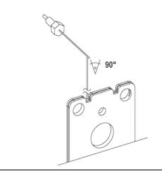
**10** The capillary lays in the grove and should be tied around the body (in the grove) 5 times.
