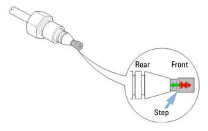
Figure 106 Capillary fitting
