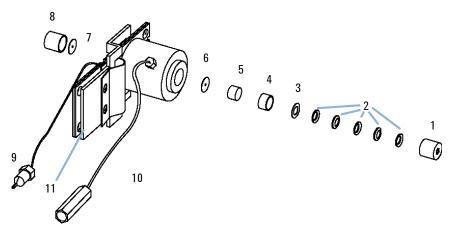
Figure 69 Semi-Micro Flow Cell Parts
