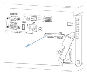
Figure 63 Replacing CompactFlash card
