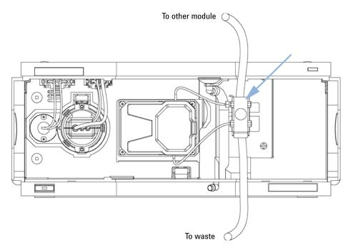
2 If it is desired that the system has only one leak drain tube, then it's possible in increase the length of the small plastic tube which is connected to port# 4 of the sampler switching valve. This tube can then be taken to waste separately. The tube which normally serves as the detector cell outlet tube can be used for this purpose.
