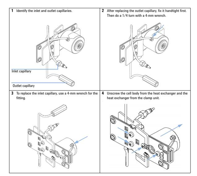
Replacing Capillaries on a Semi-Micro and Micro Flow Cell
