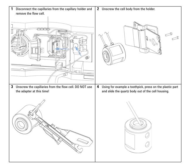
Nano Flow Cell - Replacing or Cleaning
