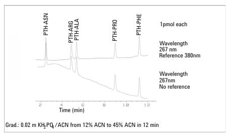
Figure 37 Gradient Analysis of PTH-Amino Acids (1 pmol each), with and without Reference
