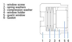
Figure 66 Orientation of Spring Washers
