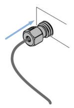
**3** Finger tighten the nut into the port until snug.
