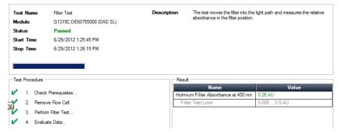
Figure 47 Filter Test
