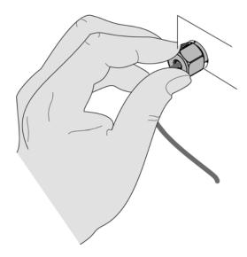
**4** Use Fitting mounting tool (5043-0915) or a 5 mm hex wrench for fixing the fitting (maximum torque 0.8 Nm).
