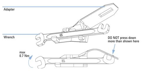
Figure 60 Wrench plus Torque Adapter
