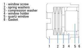
Figure 70 Orientation of Spring Washers
