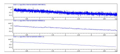
Figure 34 Influence of Response Time on Signal and Noise
