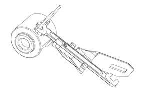
10 Reassemble the flow cell body to the holder.
