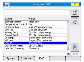
Figure 105 Instant Pilot - LAN Configuration
