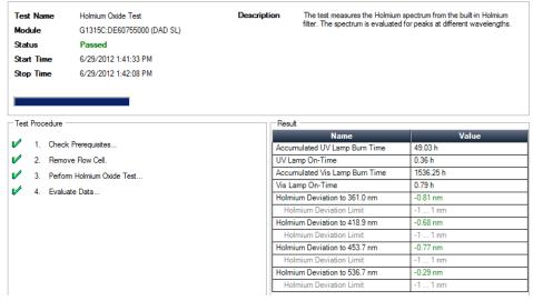
Figure 51 Holmium Oxide Test
