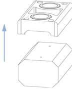
7 Replace the cell seal assembly onto the quartz body. Always use a new seal assembly to exclude damage
