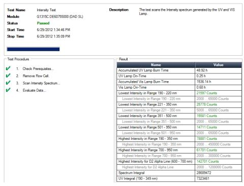
Figure 49 Intensity Test
