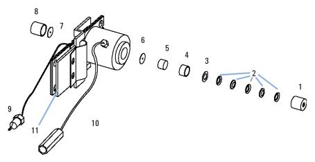
Figure 71 Micro Flow Cell Parts
