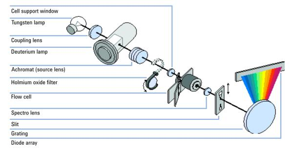
Figure 1 Optical System of the Detector
