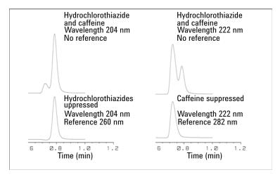
Figure 41 Peak Suppression Using Reference Wavelength
