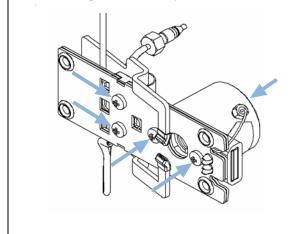
**8** Fix the inlet capillary to the flow cell body handtight first. Then do a 1/4 turn with a 4-mm wrench.
